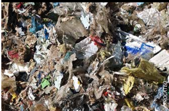
Figure 8: RDF >30mm for calciner firing
