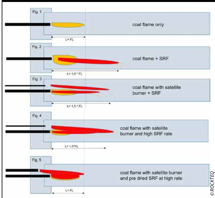
Figure 3: increased availability of oxygen by secondary air flow pattern is increasing the ignition reaction, shortening the ignition distance (pre-dried AF), accelerating the carbon burning reaction (shorter flame), minimising the tendency of particle fall-out of flame, provides higher clinker quality, maintains sintering zone length at lower kiln inlet temperature and results in less sulphur circuits
