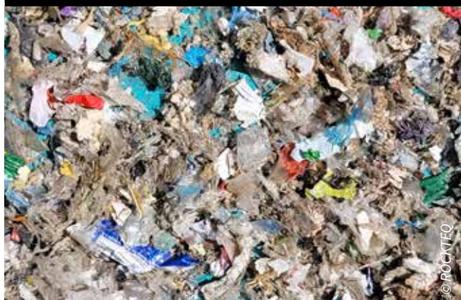
Figure 7: SRF<30mm suitable for main kiln firing
